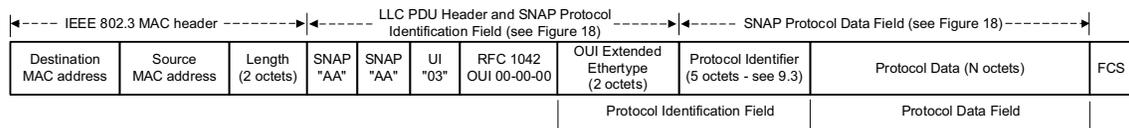
**Figure 4—802.3 frame with the OUI Extended Ethertype encoded in an LLC PDU**
