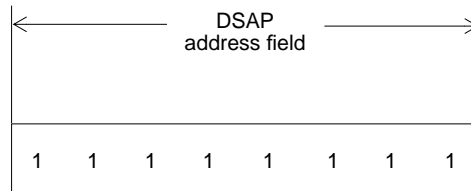
Figure 6—Global DSAP address field format
