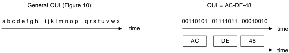
Figure 13—IEEE 802.3®, etc., frame: Order of bit and octet transmission for an OUI in a MAC address contained in a MAC Information field
