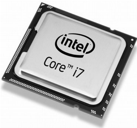
Figure 1.1 Intel Core i7 980X at 3.33 GHz (6 cores).
