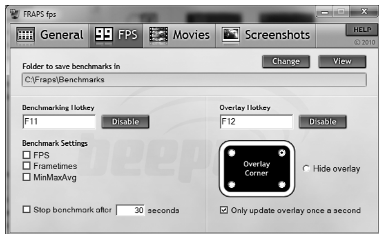
Figure 6.5 The framerate overlay options in FRAPS.
