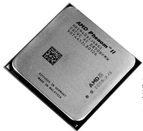
Figure 1.2 AMD Phenom II X6 1090T at 3.2 GHz (6 cores).
